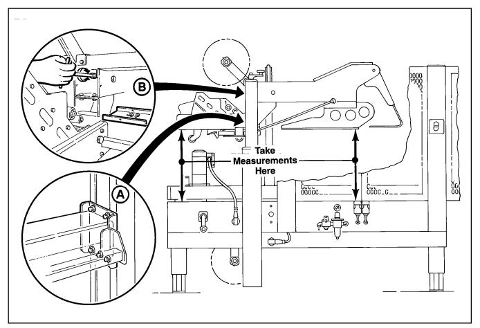
Figure 5-2 – Upper Taping Head Leveling
